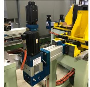
**New system: Kyntronics SHAs with "In-Line" and "Rt-Angle" Configurations**
