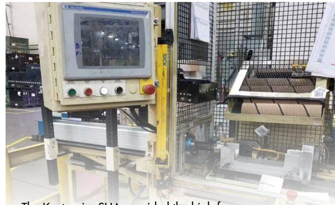
The Kyntronics SHA provided the high force required in a compact space envelope. The SHA combines the power of hydraulics with the precision of servo control resulting in a more-reliable solution for this customer while providing the position and force accuracy for repeatable quality from this assembly process.
