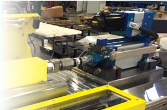
The SHA was provided with a high precision, Balluff magnetostrictive position sensor and Kyntronics fitted a customer-supplied load cell to the rod-end of the actuator. Both the position and force sensors coupled with the Kyntronics actuator controller achieved the desired accuracy and control required by this application. In addition, Kyntronics provided actuator mounting brackets for the SHA that allowed for simple installation to the test stand itself.
