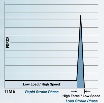
Servo-Controlled, Precise Displacement
