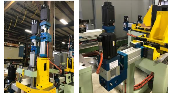
New system: Kyntronics SHAs with "In-Line" and "Rt-Angle" Configurations
