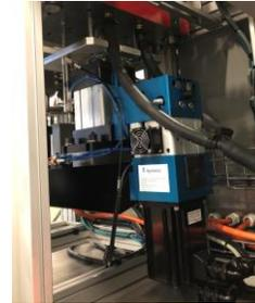
Kyntronics SHA rated at 12,100 Lbf. (54 kN) of force. Note the innovative” Inverted Parallel “configuration, a design feature unique to the SHA product.
