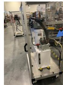
The Kyntronics SHA eliminated this HPU, and dual hydraulic cylinders used on the previous machine.
