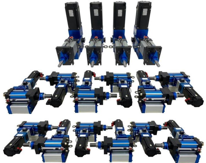
16 – SMART Electro-Hydraulic Actuators in two Configurations used on the Metal-forming Line
