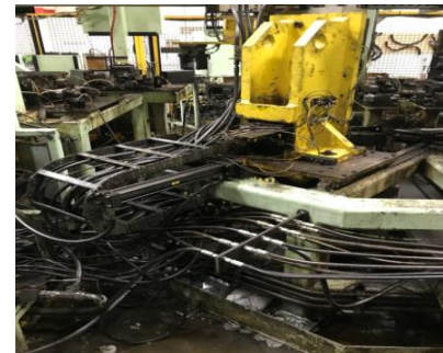
HPU-Driven cylinders have many components and connection points
